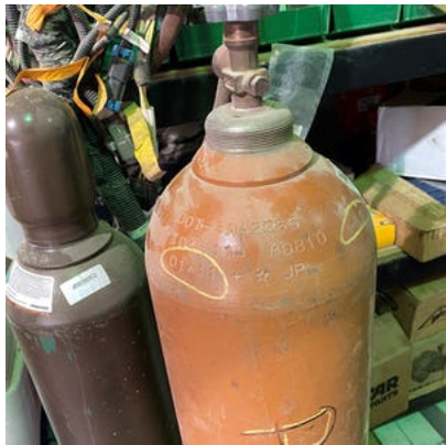
Unused cylinders not protected from falling / Unused cylinder missing cap
