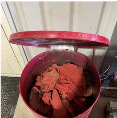
Rags stored in approved container.
