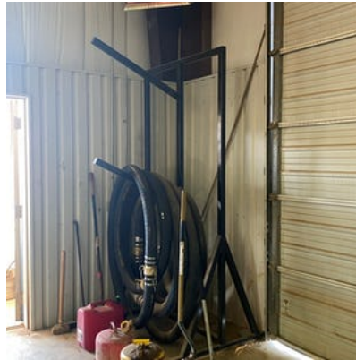
Flammable materials being stored near a heat-producing source. Moved to separate area.
