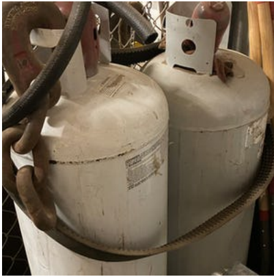
Tanks not marked noting specific product. Cylinder not protected from falling.
