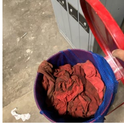
Oily rags stored in approved non-flammable container.
