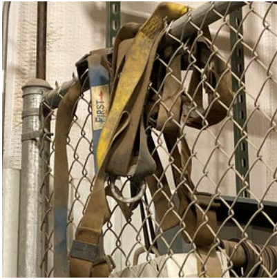
Improper storage of fall protection equipment.
