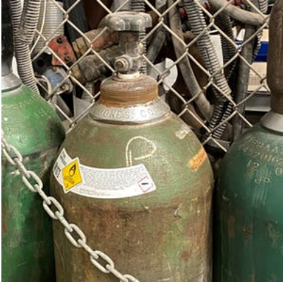
This set of cylinders has fall protection, middle cylinder is missing cap.
