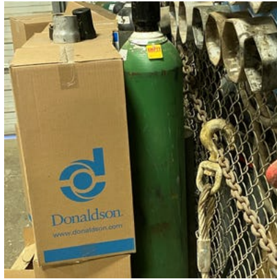
Tanks not marked noting specific product. Cylinder not protected from falling.
