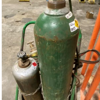
Mobile hot work equipment has proper fall protection and cylinder markings (oxidizer, flammable).
