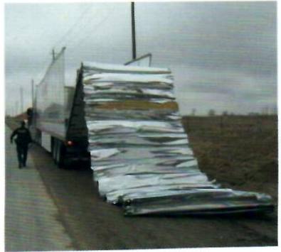
a. (3) Upper Rail with Missing Roof Bows
