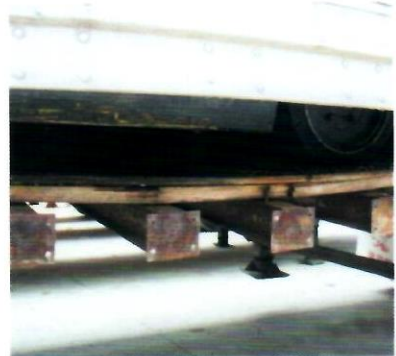
c. (1) and (2) Protruding Freight and Sagging Crossmembers
