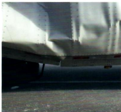
b. (1) Broken Lower Rail
