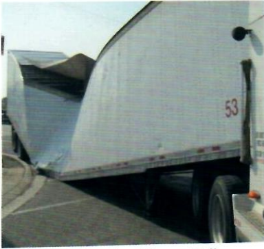
a. (1) Broken Upper Rail b. (1) Broken Lower Rail
