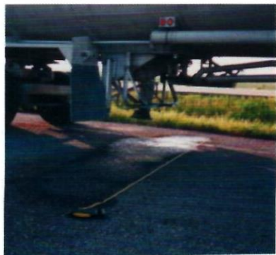
e. Leaking Cargo Tank
