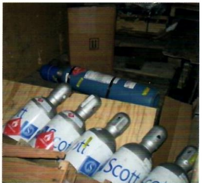
a. HM/DG Not Properly Secured
