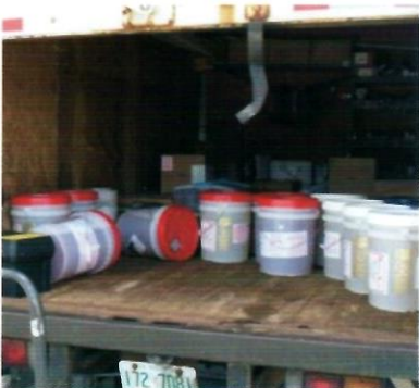
a. HM/DG Not Properly Secured
