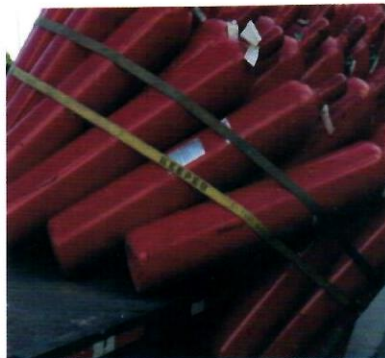
a. HM/DG Not Properly Secured
