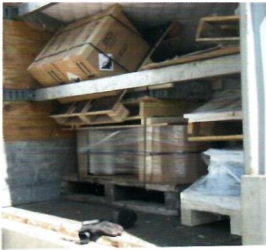
a. HM/DG Not Properly Secured
