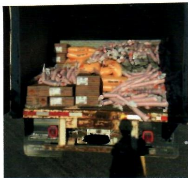
a. HM/DG Not Properly Secured
