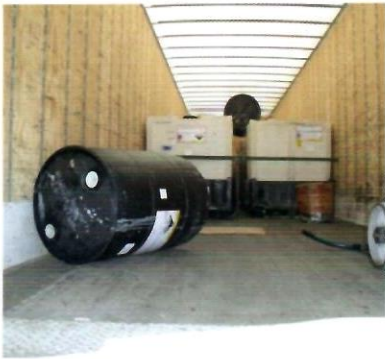
a. HM/DG Not Properly Secured
