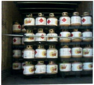
a. HM/DG Not Properly Secured
