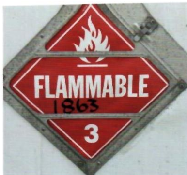
a. Inappropriate ID Marking
