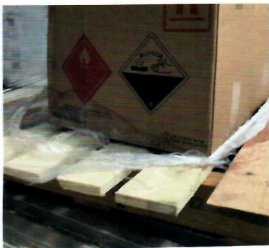
HM/DG Leaking from a Package
