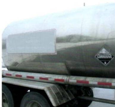
a. (1) Missing ID Number (4 sides)
