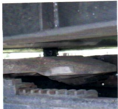
b. (3) Kingpin Not Properly Engaged
