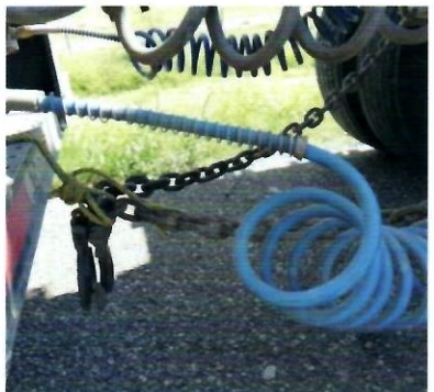
f. (2) Improper Connection
