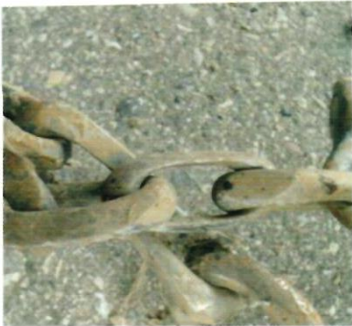
f. (4) Excessive Wear
