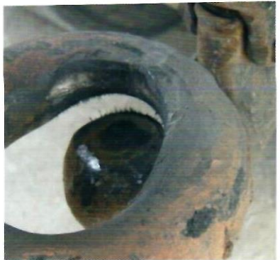
d. (4) More Than 20% Reduction in Drawbar Eye
