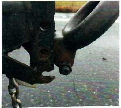
d. (2) Ineffective Fastener
