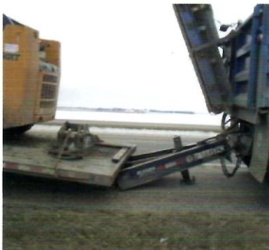
e. (2) (a) Cracked Drawbar
