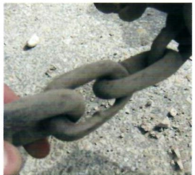
f. (4) Excessive Wear
