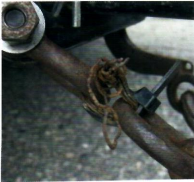
f. (3) Improper Repair
