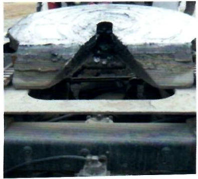
a. (3) (b) Aft Stop Missing
