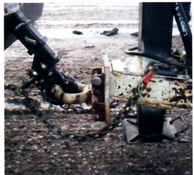
c. (1) Loose Pintle Hitch Mounting
