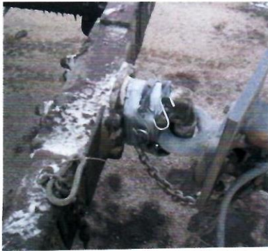
c. (1) Insecure Pintle Hitch Latch
