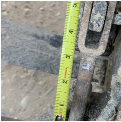
Axle 1 Left - Steering brake out of adjustment - Type 20 Clamp (2 1/2" stroke) - 2 3/4 measured
