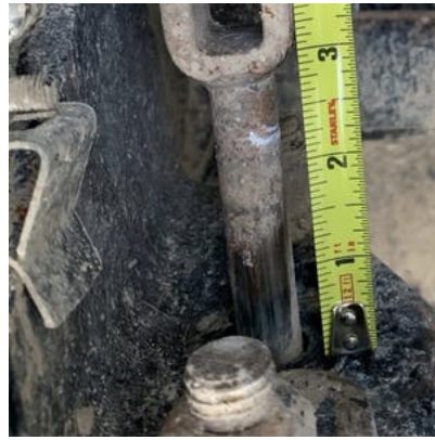
Axle 1 Right - Steering brake out of adjustment - Type 20 Clamp (2 1/2" stroke) - 2 1/4 measured
