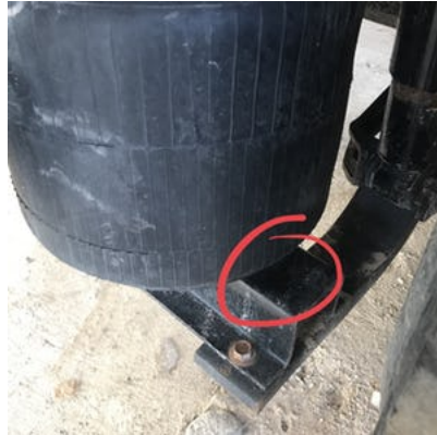
Axle 3 right side air bag leaking at the bottom near crossmember.
