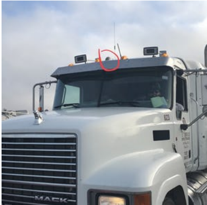
Missing center ID lamp
