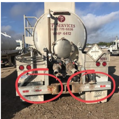
Bumper reflective sheeting torn / faded
