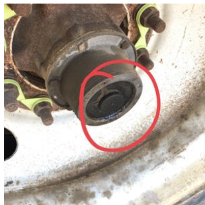
Axle 5 right side, oil residue on hub cap
